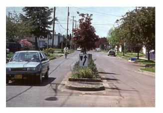
• **Bulbouts** are appropriate at locations with usable space next to the curb. Consider bulbouts at intersections of three or more lanes. Bulbouts should not extend further than six feet into the street adjacent to parallel parking, or 12 feet adjacent to diagonal parking. At locations with no on-street parking, bulbouts should not impede bicycle travel.
