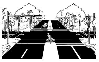
• Split Pedestrian Crossover (SPXO) – The SPXO is a pedestrian refuge that channels pedestrians, using railings, to cross one half of the street; enter the island at one end; walk towards the flow of traffic; and exit at the other end to cross the second half of the street. SPXOs can improve pedestrian safety
