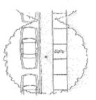
Continuous sidewalks, separated by a planter or park strip with a vertical curb, create a pedestrian-friendly environment.
