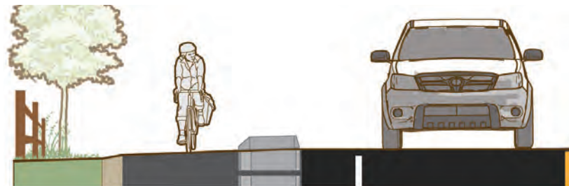
Figure 4-19. Separated bike lanes may be configured on an existing roadway surface by using a physical barrier such as a curb or median to separate the bikeway from the roadway.
